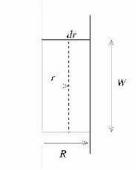
Consider a small strip of length W and width dr that is a distance r from the axis of the wire. The flux through the strip is
